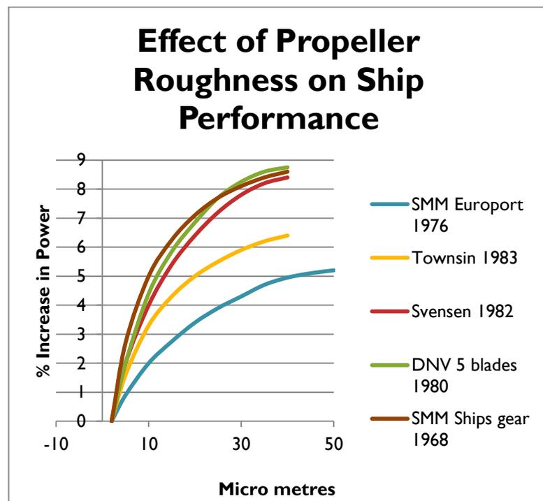
More recently many other experts and authorities have been investigating the effect of roughness. Much of this work deals with the varying effects of different types of propeller roughness, including the average slope of the roughness profile and other texture parameters as distinct from the average height of the roughness. This is very
